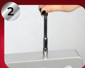
2 Tighten the screws to panel device securely with a socket
